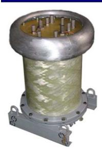
Separately mounted gas-filled current transformer (TOG-35-II) is designed for application as a mean of verification of industrially produced current transformers, can be used for transmission of the measuring information signal onto the measuring instruments during high-voltage tests of electrical equipment.
